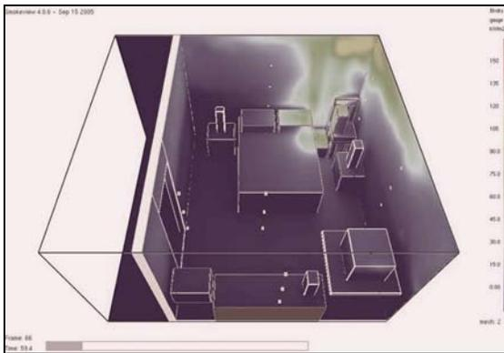
Fig. 1 - Wall heat flux 2.5 min before flashover
