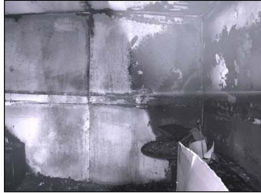
Fig. 6 - Photo panorama of wall opposite open doorway. Note similarities of clean-burn to areas of high heat fluxes shown in Figs. 4 & 5
